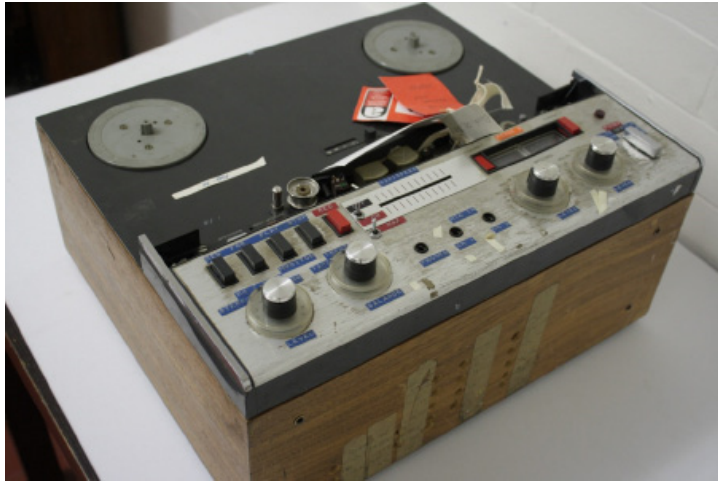
Figure 6. Revox A77 tape recorder modified by Hugh Davies. The vari-speed modification is a clue that this example was used creatively, as part of an electronic music studio or live on stage. Science Museum, London, object no. 2007-136.
