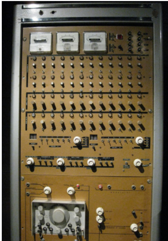
Figure 4. Analogue sequencer by Landrieu and Goethals. Musical Instruments Museum, Brussels, inventory no. D1999.002-03.
