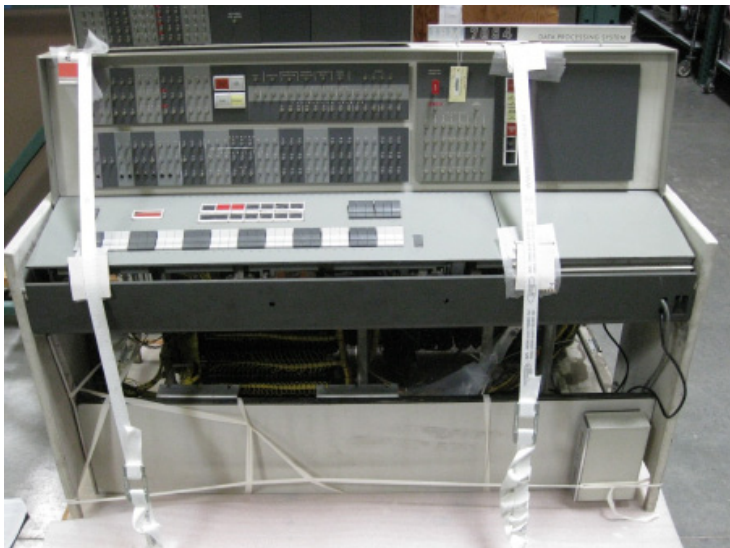
Figure 2. Console control unit for IBM 7094. A system of this kind was placed in service at Bell Labs in 1964, superseding the IBM 704 and 7090 systems. Mathews and his team had to rewrite the MUSIC programs for each new system. Computer History Museum, Mountain View, CA. Paul Pierce Collection, lot no. X7021.2014.
