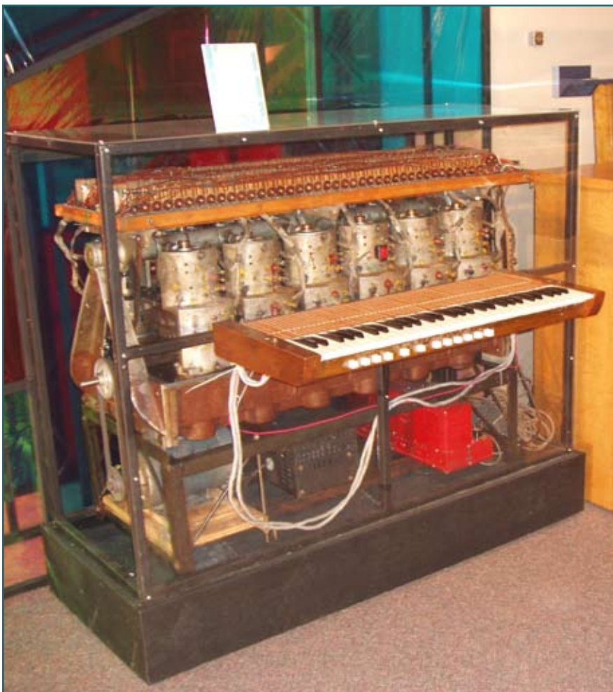
The Robb Wave Organ, a 1930s tone-wheel electronic organ by Canadian inventor Frank Morse Robb.
