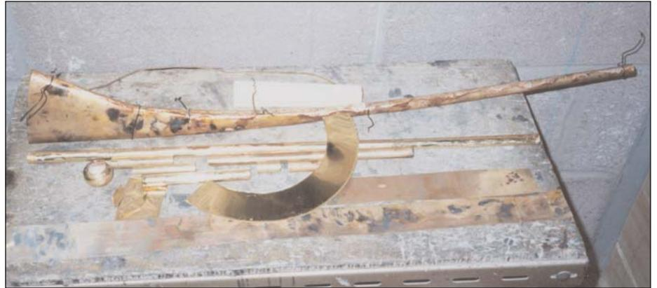
Figure 1. The trumpet in progress: the bell after soldering before hammering and burnishing, tubes, the ball, sheet brass for the garland and some more tubes, the wooden block, and wire for the rim.
