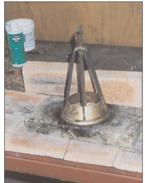
Figure 3. Fitting the wire rim to the garland.
