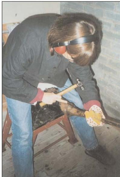
Figure 2. Hammering the bell on an anvil.
